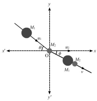
Initially mass  $M_1$  is moving with velocity  $u_1$  at an angle  $\theta\theta$  with x-axis and the mass  $M_2$  is moving with velocity  $u_2$  along the x-axis.
